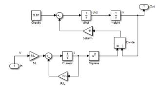
The Magnetic Ball Plant model represents an iron ball of mass M. This ball moves under the influence of the gravitational force, Mg, and an induced magnetic force,  $\frac{\beta i^2}{h}$ . The presence of the squared term in the induced magnetic force results in a nonlinear plant.
